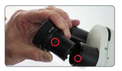
If you wear eyeglasses for microscope viewing, keep the rubber eyeguards folded down. If you do not wear eyeglasses, you may find it useful to unfold the rubber eyeguards in order to block out ambient room light.
